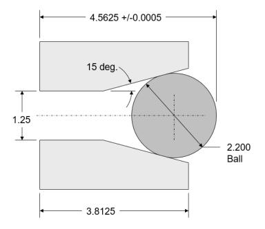
The problem is compounded because this dimension has a very tight tolerance. Several sizing adjustments may be required during a cutting tool's life as the tool wears.
