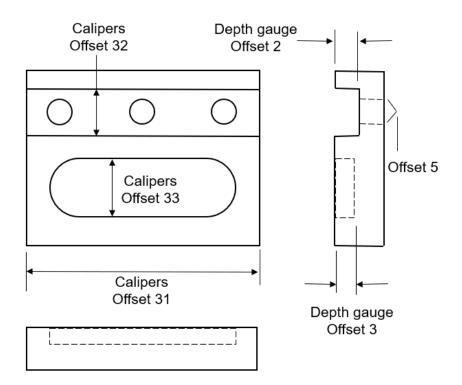
We're showing a machining center application, the same techniques can be used for turning center applications. Notice that every machined surface is documented. This documentation names the gauging tool must be used to measure each workpiece surface, as well as the offset number that must be adjusted when sizing is required.
