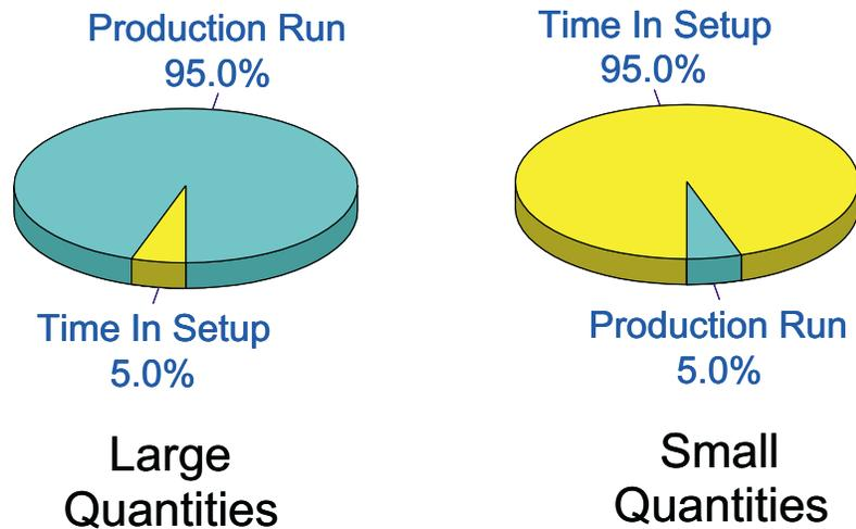
The larger your lot sizes, the greater the percentage of time that the machine will be in production and the fewer the number of needed setups. With very high production quantities, a very small percentage of the machine's overall time will be spent in setup. There are CNC machines, in fact, that are dedicated to running only one workpiece - day in and day out. Once the job's setup has been made once, the machine will never be in setup again.
